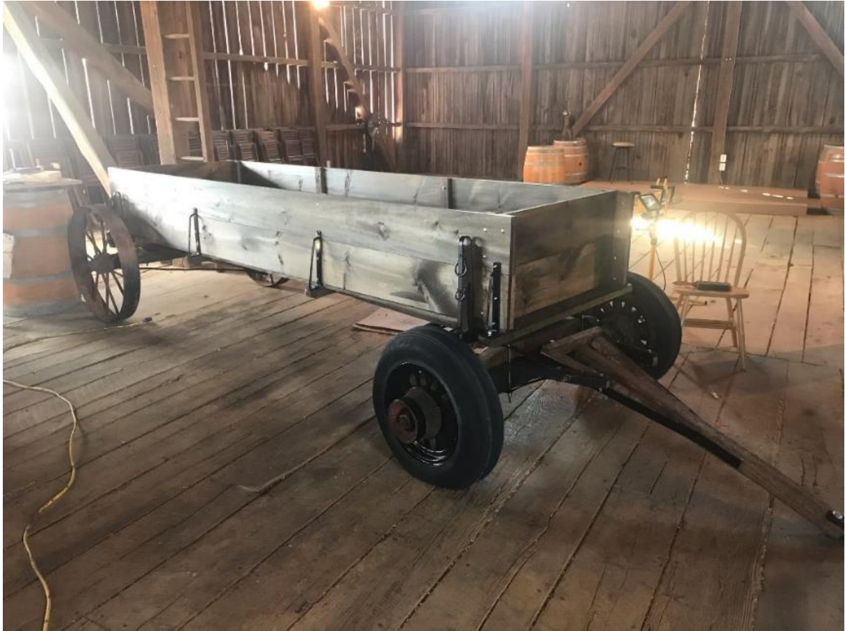
Wagon bed assembled and stained with temporary iron wheels still on the back.
