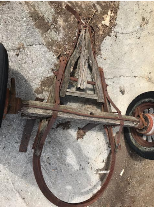
Original Front Axle with Tongue
