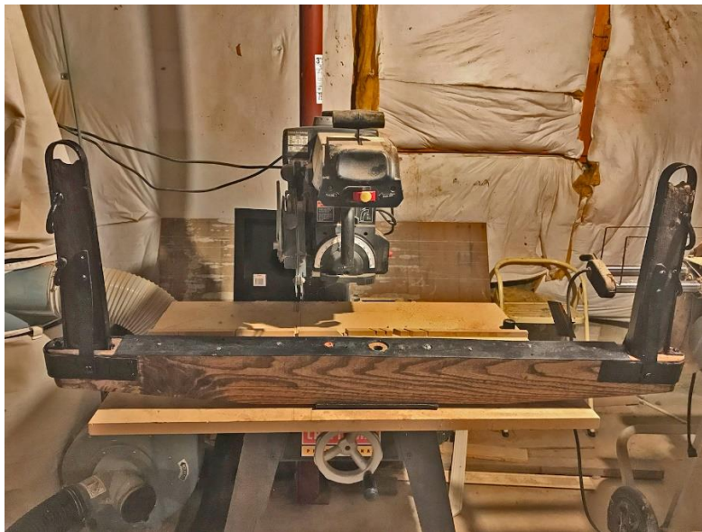
New Front Bolster with reused bolster stakes and hardware attached.
