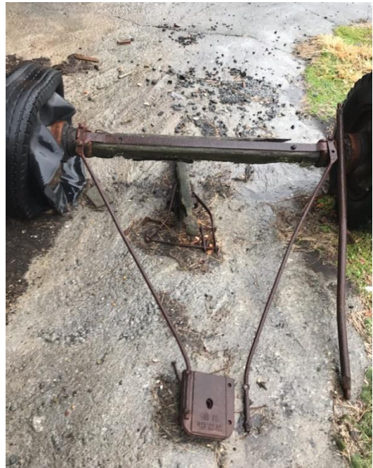
Original Rear Axle with Reach Plate
